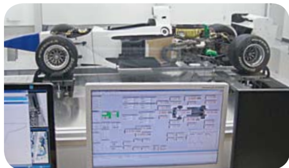
Servotest four, six and seven poster vehicle test rigs
