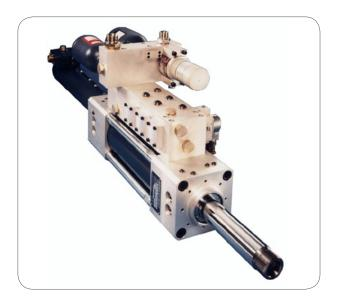
A pressure accumulator is fitted close to the servo valve pressure port to provide instantaneous flow to meet peak demands. There is also an exhaust accumulator close to the servo valve exhaust port to smooth pulsations in the return line.
