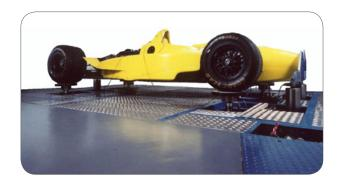
Servotest have now delivered some sixteen 7 post race car simulators, eleven of which were destined for F1 GP teams. A recent major step forward was replacing the DCS2000 control system with the latest state-of-the-art fibre-optic linked PULSAR controller. A very comprehensive RACECAR software suite has been developed, with continual feedback from our customers to push the performance envelope of the rig.
