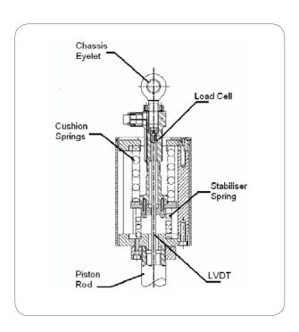
Servotest's solution to this problem consists of an aluminium cylinder, containing a link assembly suspended by two preloaded coil springs, each of different stiffness. The cushion spring helps to simulate the progressive effect of the car suspension under compression, whilst the stabiliser spring simulates extension and provides pre-load.
